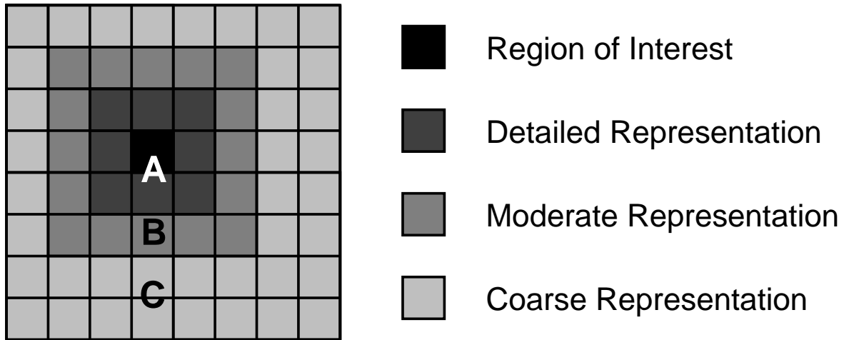
Figure 11: Specific approach: the problem is broken into 2^{d(\bar{m})} pieces on scale \bar{m} , where \bar{m} is selected to keep the size n2^{-\bar{m}} of each piece constant, independent of total problem size n . Each piece A is surrounded by two concentric bands of decreasing statistical detail \zeta_A, \zeta_B , followed by a coarse representation C of the remaining domain.
