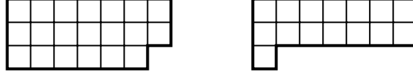
Fig. 4. Boundary length problem: both regions have the same boundary length, although very different volumes.
